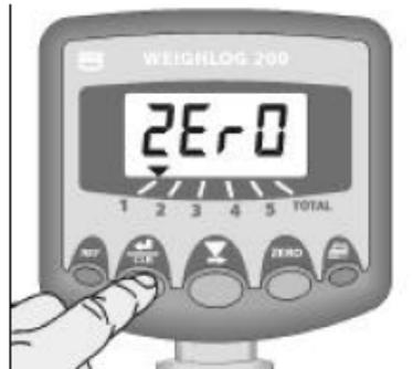
Figure 23 : Proportional Scaling ("ZERO" routine)
