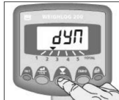
Figure 5 Select Weighing Mode
