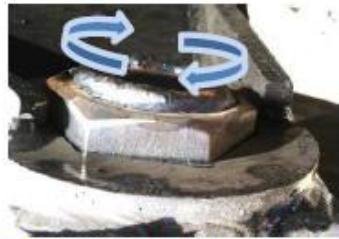
Weld O.D. of bolt shank to I.D of hex nut
