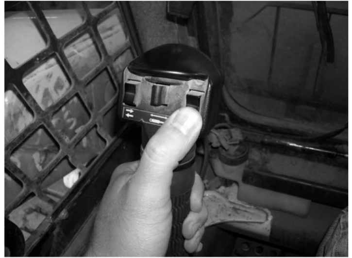
PUSH AND HOLD TO ENERGIZE DIVERTER
