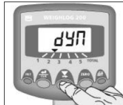
Figure 5 Select Weighing Mode
